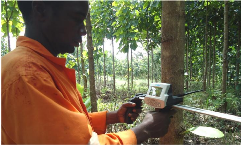
Figure 3: Diameter at Breast Height (DBH) measurement being conducted using MasserCalliper during an enumeration exercise
