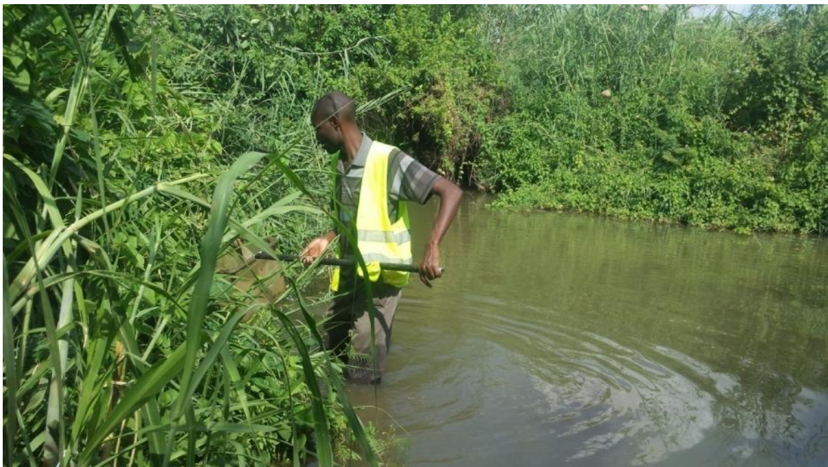
Figure 6: Mini-SASS river sampling being carried out on Mafinji River
